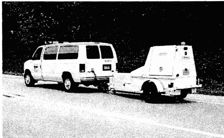
Photo 13. Another View of VDOT's Falling Weight Deflectometer. Note the load pad in contact with the pavement surface at the rear.
