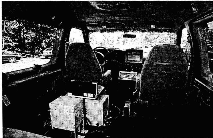
Photo 5. Profiler's On-Board Data Acquisition System
