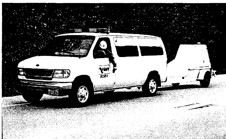
Photo 12. VDOT's Dynatest Falling Weight Deflectometer. The operator is measuring the surface temperature with an infrared gage.
