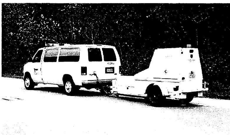
Photo 13. Another View of VDOT's Falling Weight Deflectometer. Note the load pad in contact with the pavement surface at the rear.
