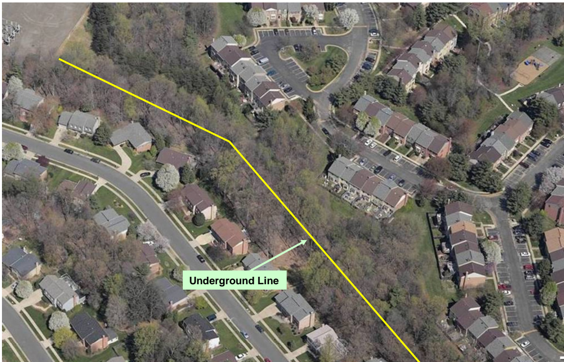
Figure 20: Underground 230 kV Line in Fairfax County Was Built Because Rapid Development Eliminated Viable Overhead Route
