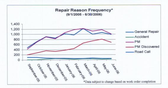
Trends to take note of in the above table are road call and PM discovered repairs. It is the VMCC's goal to keep the road call repairs to a minimum. Although most are unavoidable, many road calls can be avoided by catching the problem early. The more repairs that are found during a PM Service, the less likely a vehicle will breakdown and require an unscheduled repair. Note road call line trending down as PM Discovered trended upward until leveling then falling.
