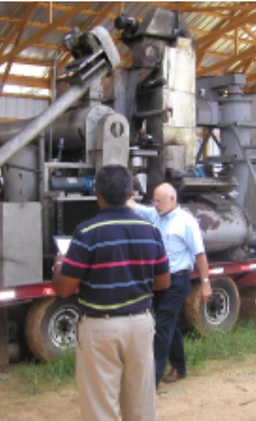
A Special Projects grant is funding the construction of next generation pyrolysis units to demonstrate the conversion of wood chips and other plant material to bio-diesel crude oil.
