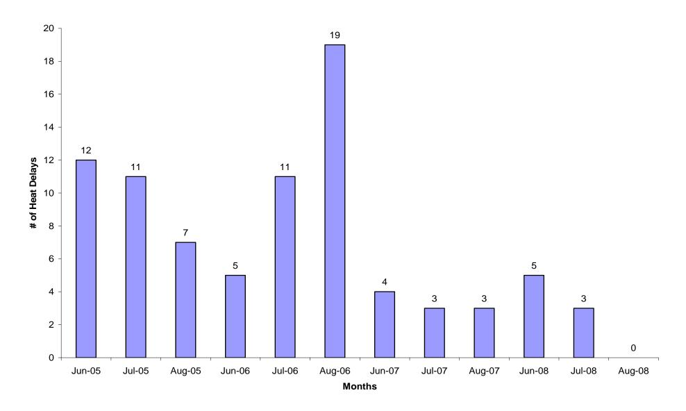
The intent is to increase safety during operations in hot weather that might cause continuous welded rail to bend or kink as a way of relieving pressure. CSX issues heat orders along the railroad's entire system, including track from New England to Florida.
