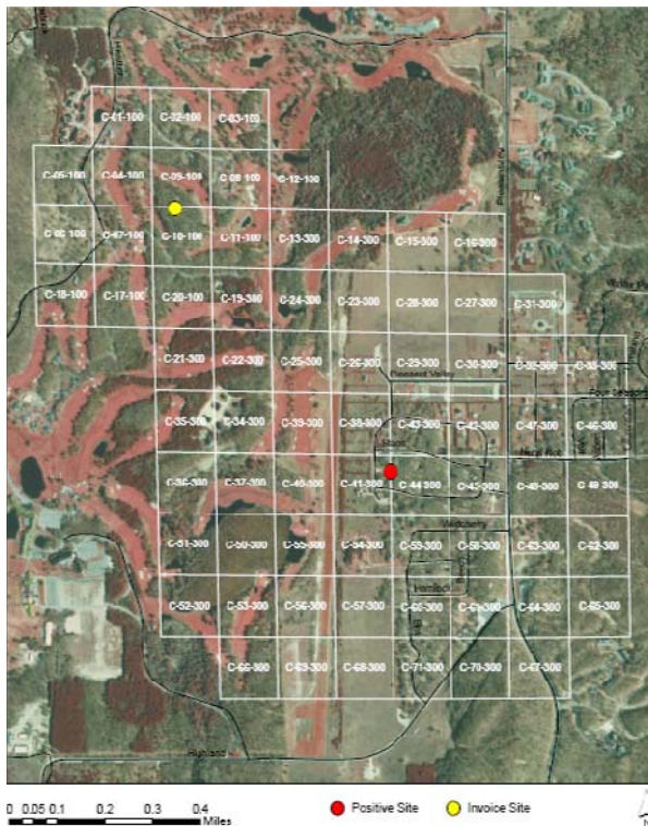
Figure 3. Example of a map utilized by field staff to conduct surveys around positive and invoice sites using ten-acre plots defined by Public Land Survey System quarter-quarter-quarter sections. In addition to carrying paper maps for navigation, surveyors were electronically “tethered” to GPS coordinates corresponding to the centroids of each plot to ensure that they remained within a given plot while it was being surveyed.
