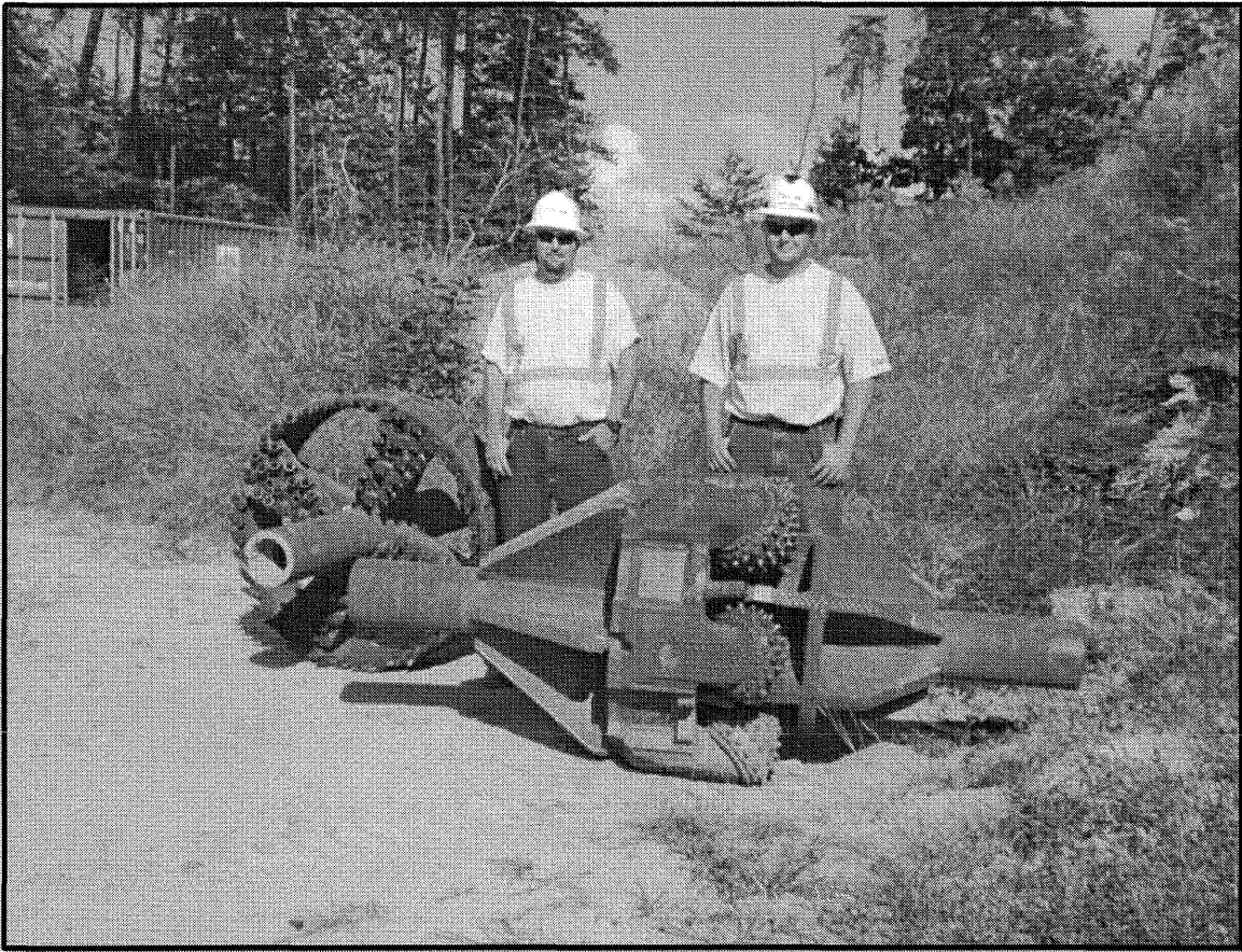
Figure 4: 42-Inch Drill Bit (Reamer).
