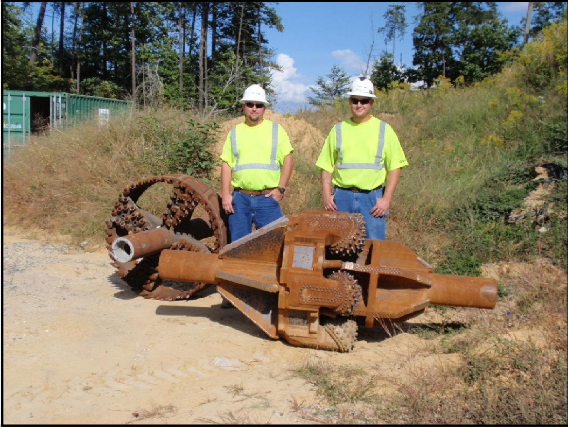
Figure 8: 42-Inch Drill Bit (Reamer).
