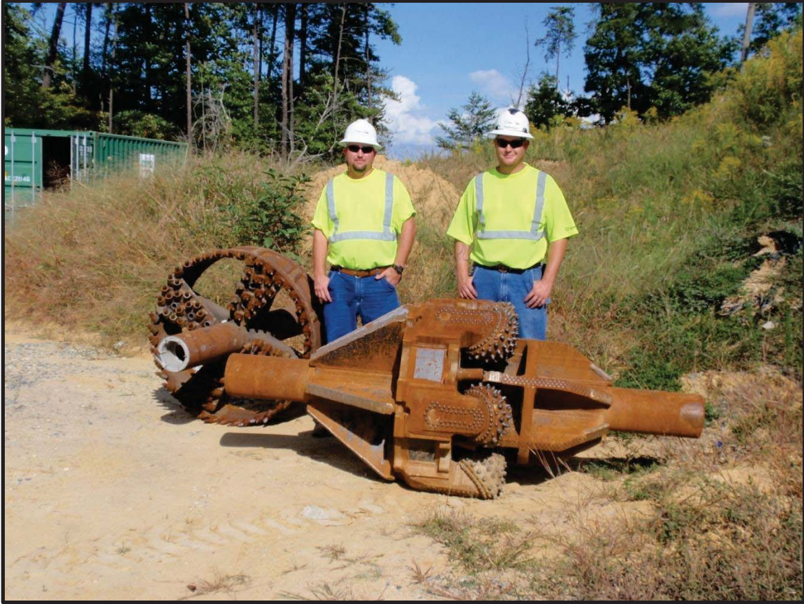
Figure 8: 42-Inch Drill Bit (Reamer).
