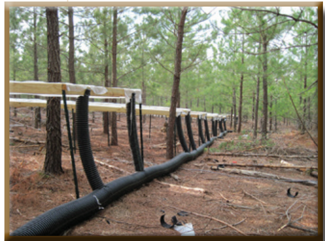
Rainfall exclusion devices on the PineMap project location at Appomattox-Buckingham State Forest studying the responses of loblolly pine to simulated drought and fertilizer additions.
