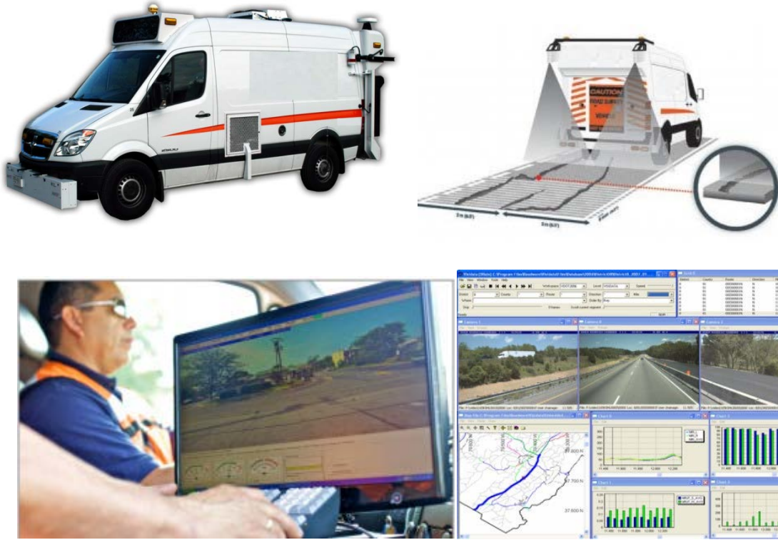
Figure 5: How Pavement Condition is Assessed
