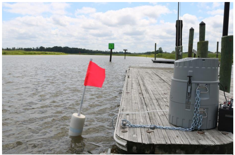
Figure 3: DSS marine science automated water sampler deployed in the Western Branch of the Nansemond River to investigate bacterial contamination and transport in the shellfish growing area.
