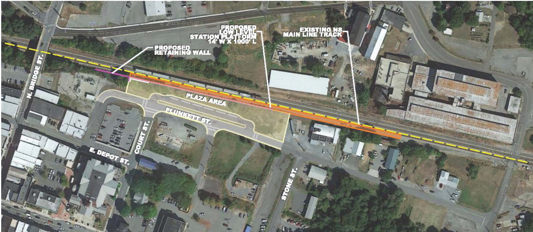
Figure 12: Rendering of 1000 foot low level platform (Town of Bedford's Locally Preferred Site)
