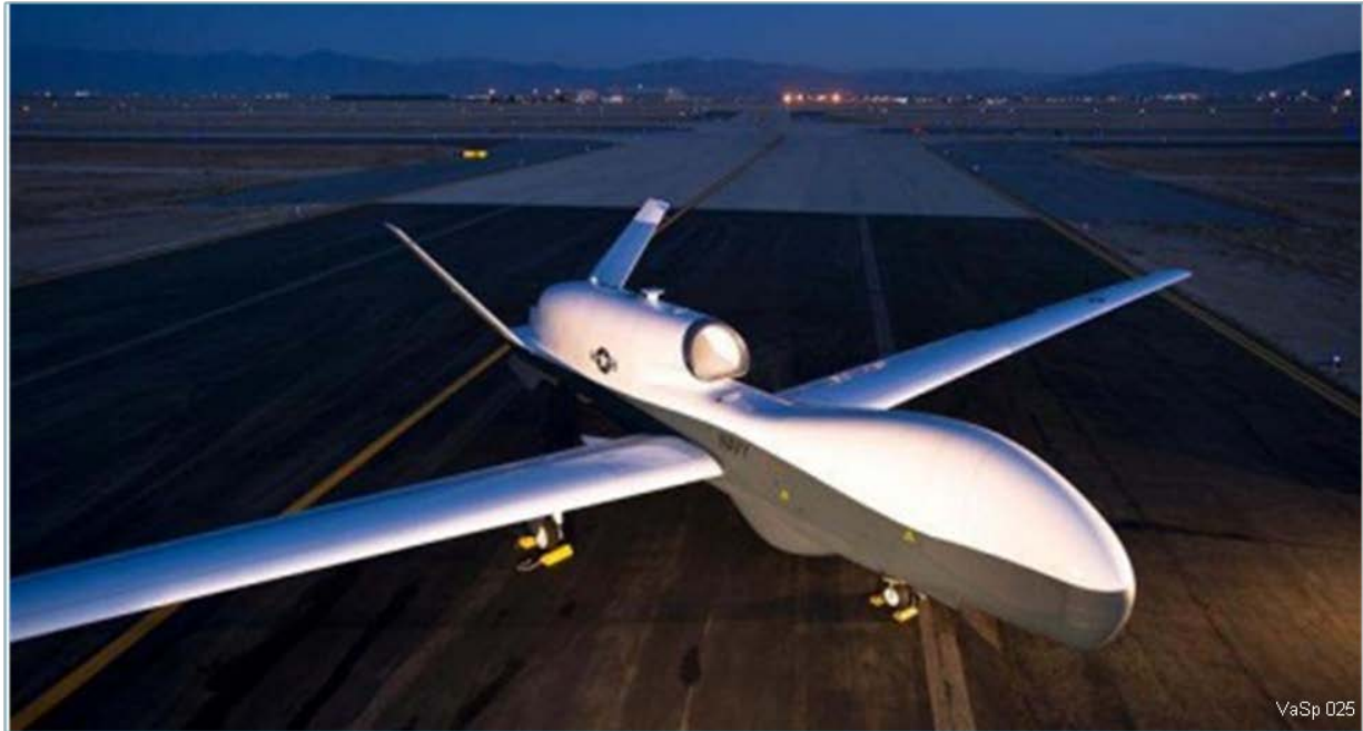
Figure 5-17. US Navy Triton UAS. The US Navy is gearing up for the first test-flight of its MQ-4C Triton aircraft, a wide-spanning 47-foot long surveillance drone. (Photo; US Navy).
