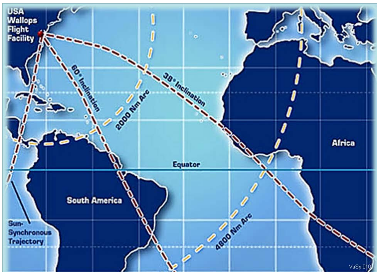
Figure 5-1. MARS Launch Trajectories. Vehicles launched from MARS can fly to a wide variety of orbits, increasing the number of potential launches the site can attract.
