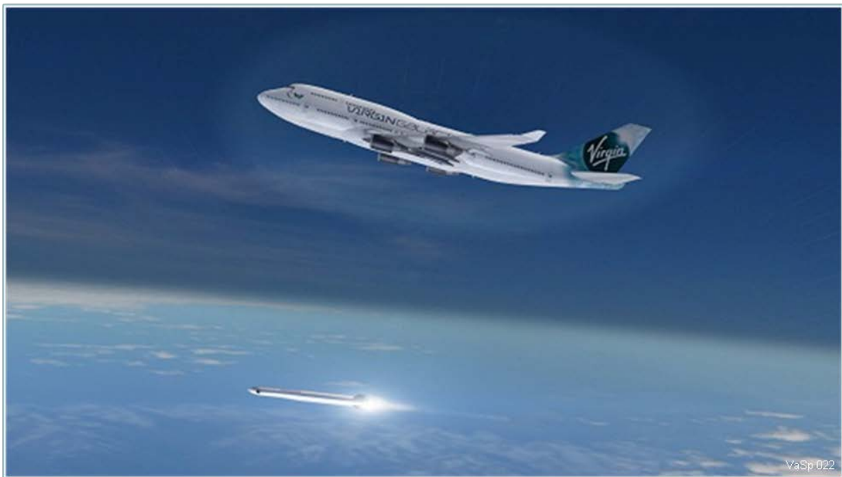
Figure 5-14. Virgin Galactic LauncherOne. LauncherOne ignites after being released from Cosmic Girl, a 747 that could take off from Virginia Space's runway. (Image: Virgin Galactic).
