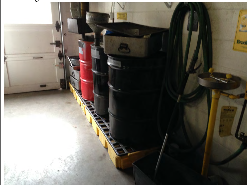
Photo 37-2 Used motor oil drums on spill pallets within vehicle maintenance bays in Building 50
