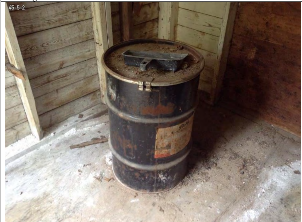
Photo 36-2 33-gallon drum of unknown chemical. Label indicates a vinyl based asphalt patch, but observed chemical spilled is an off-white powder
