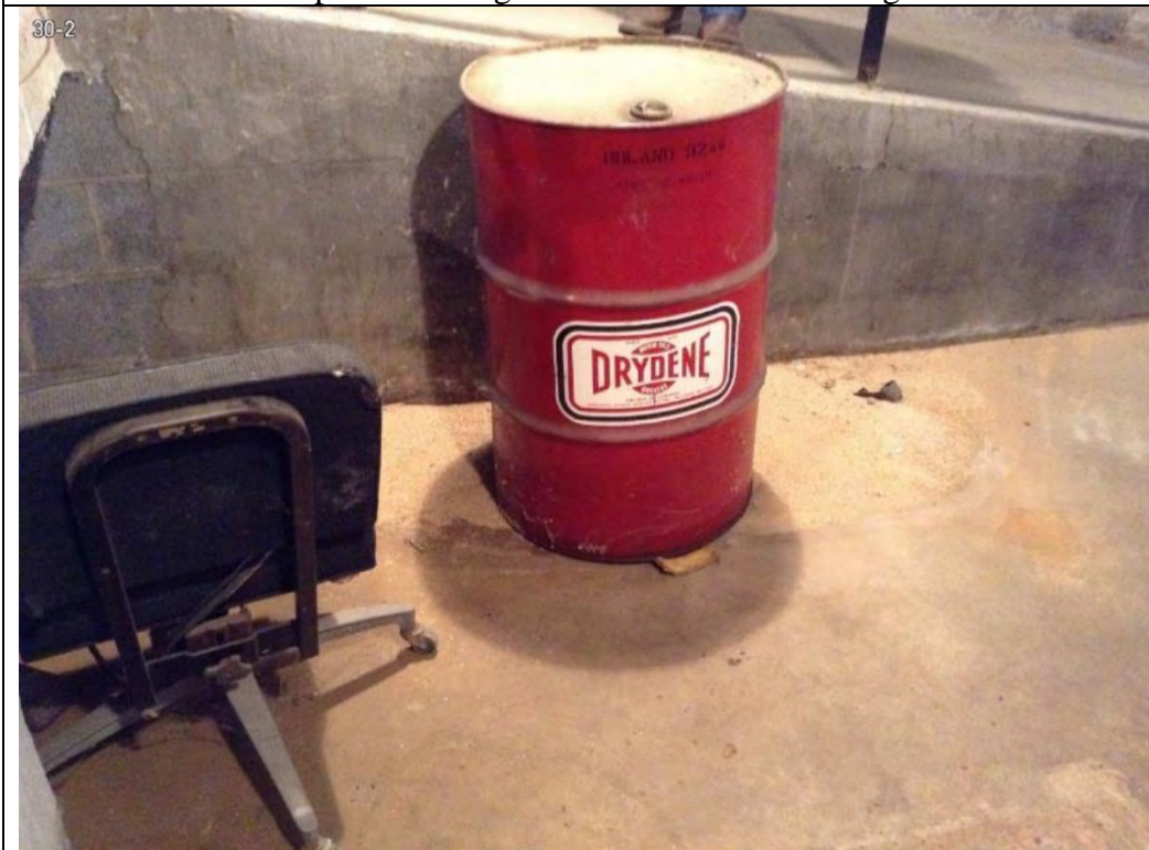
Photo 38-2 55-gallon drum of air compressor oil: Roland 32-weight Anti-Wear (AW) by Drydene Oil Company. Drydene was purchased by Castrol in 1991, thus this drum is at least 26-years old. Some indication of minor spills associated with this drum, as evident by oil-dry on floor.
