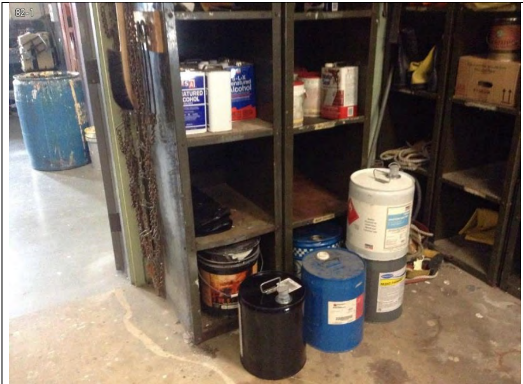
Photo 8-2 Paint thinner and solvent storage within Building 82. No evidence of spills or staining, and no floor drains present within building.
