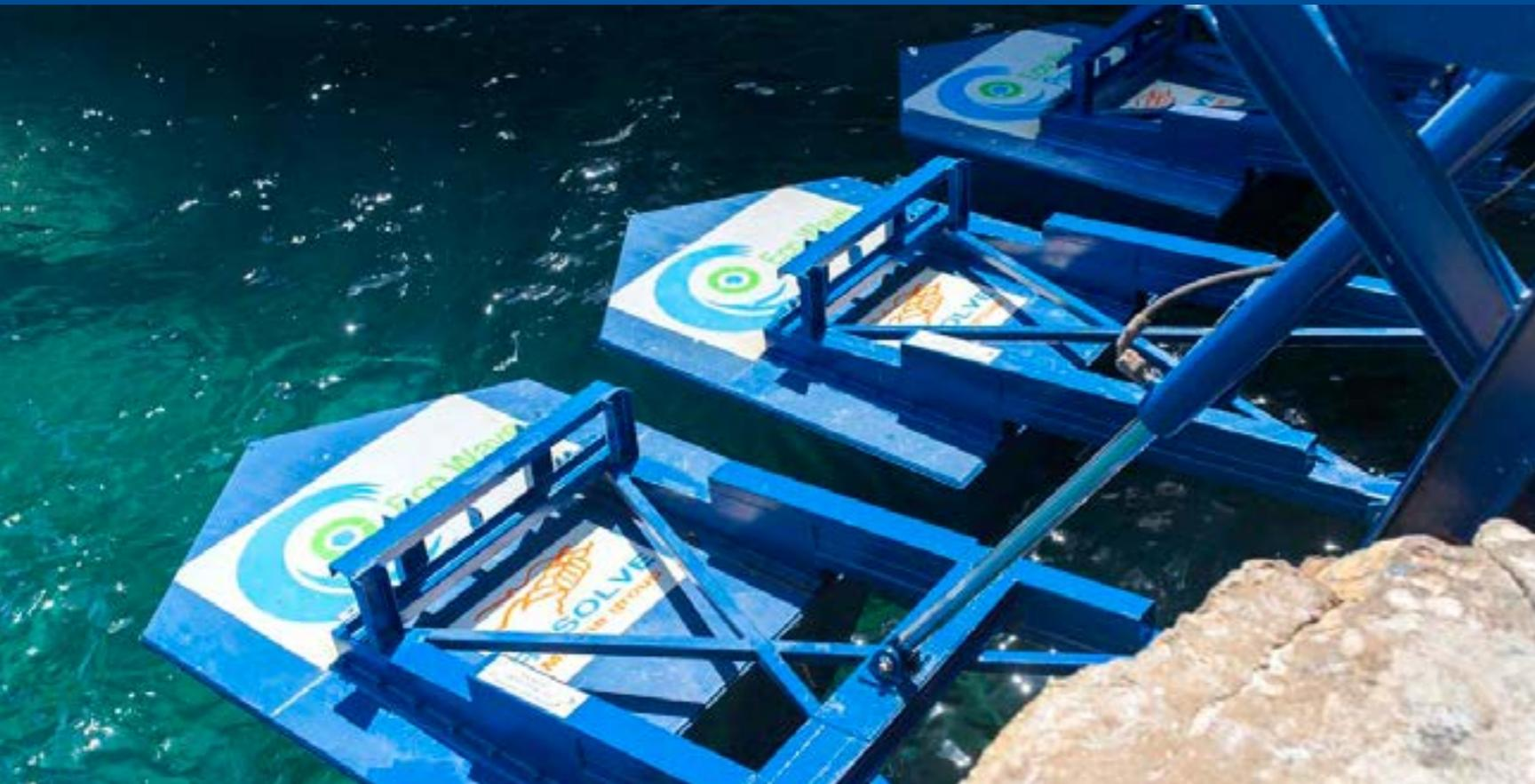
EcoWave Power – converts sea waves to electricity. The VIAB is discussing building trial power stations with sea facing counties and to base EcoWave floats on area bridges to generate electricity.
