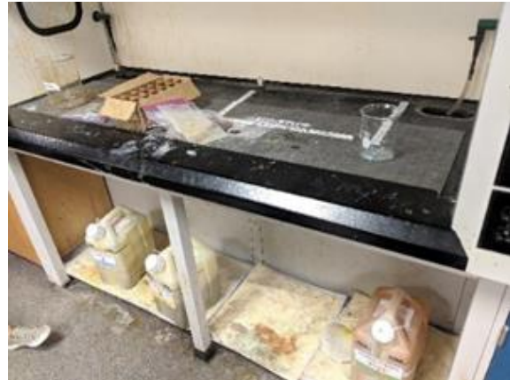
Top photo: Different shelves represent different types of chemical waste generated. Bottom photo: Waste was stored under the teaching lab fume hood at the point of generation on absorbent mats.
