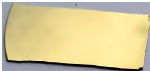
Figure 2.33: Titanium nitride thin films grown on sapphire.
