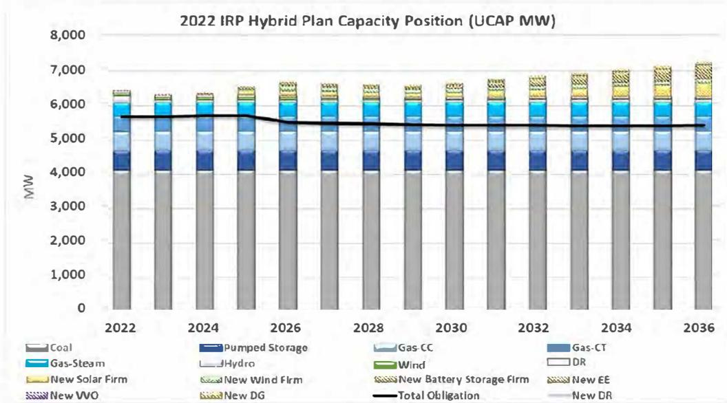
Figure 25. APCo Capacity Position with Hybrid Plan Additions
