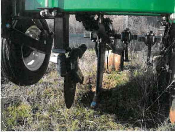
FIG 3 – Close-up of no-till ripper used to loosen subsoils after mine soil reconstruction. This implement can be pulled through existing vegetation with minimal disturbance and is used in a post-mining context when subsoil compaction is believed to be limiting productivity (photo: C Zimmerman).
