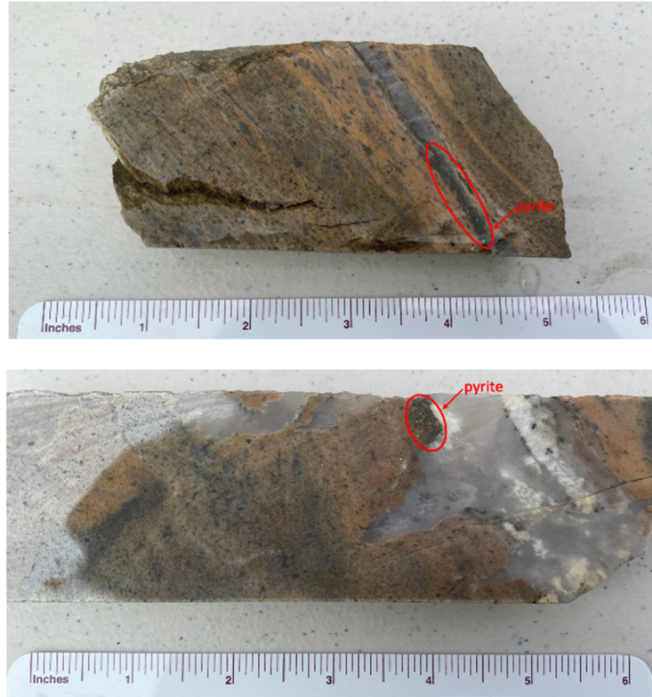
FIGURE 2-9 Photos of the Vaucluse core shown to the committee in Charlottesville on March 30, 2022. The core was collected from beneath the deepest parts of the deposit that were mined. Note the pyrite-rich areas at the quartz vein–wallrock contact. Most of the gold in these samples is contained in the pyrite. SOURCE: Photos by Robert J. Bodnar.
