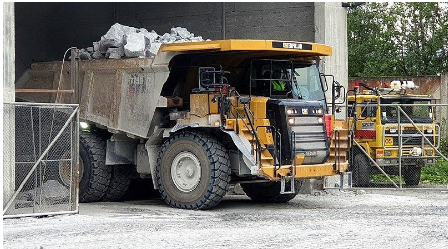
FIGURE 3-6 A 64.6 metric ton haul truck. The truck contains large blocks of rock collected from the open pit after blasting and is preparing to dump the large rocks into a crusher that will break the rocks into smaller pieces for further processing.
