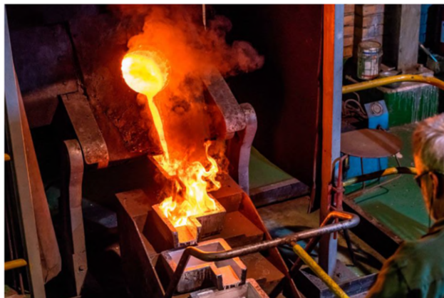
Image of gold-rich metal being poured from a refining furnace from Schoemaker (2022)
