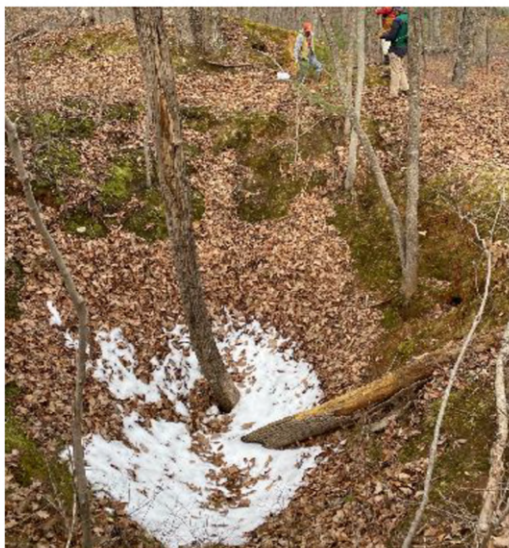
The surface expression of a shaft used to access underground ore Photo by Bob Bodnar
