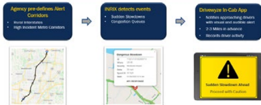
CMV Traffic Alerting - How it Works
