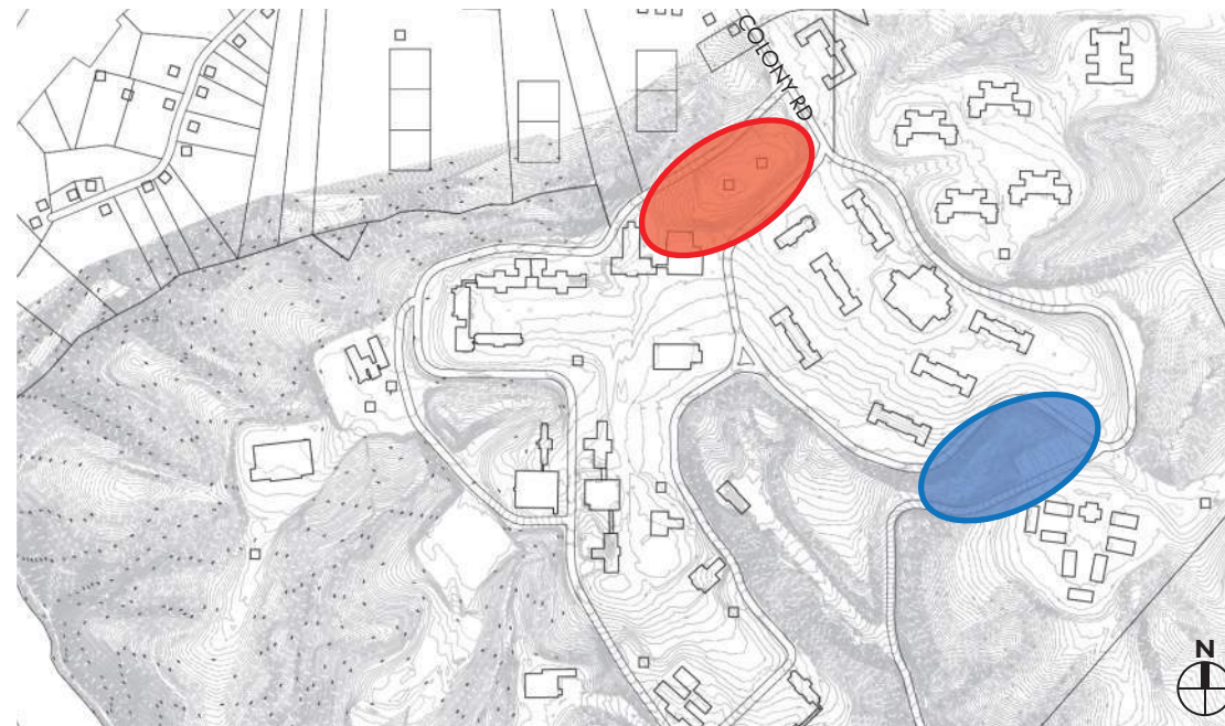
Existing Site topography showing areas that will receive major amounts of cut (red) and fill (blue) earthwork material
