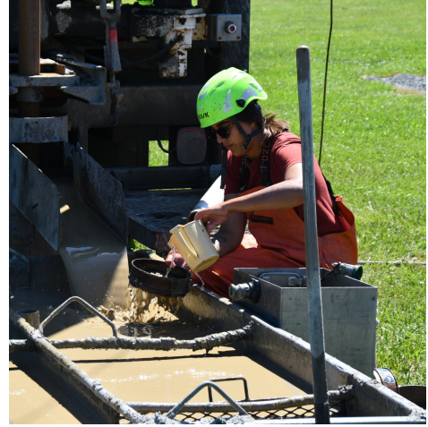
(b) DEQ geologist washing, preparing, and reviewing samples of drill cuttings.
