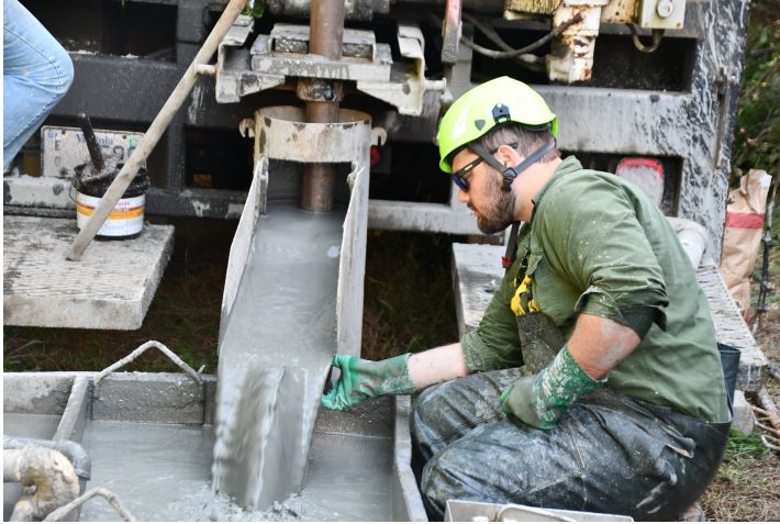
(a) DEQ geologist using a sieve to catch cuttings from mud-rotary drilling discharge.
